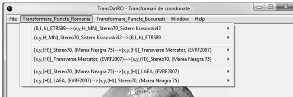
Fig. 7 – Coordinate transformations for Romania, in the TransDatRo (v4.06) application.
