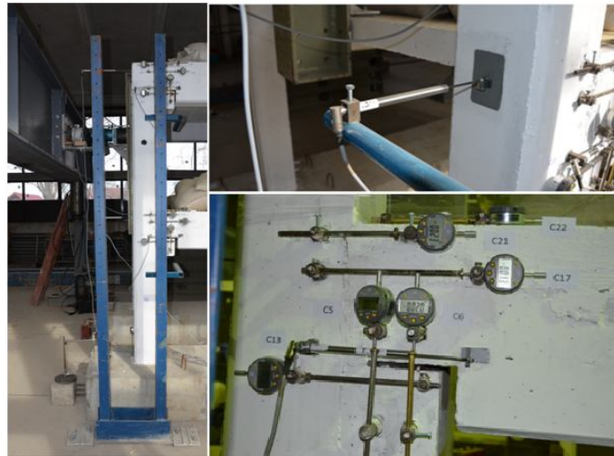
Fig. 2 – Monitoring the displacements and deformations of the structure.
